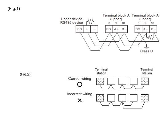
♦How to connect KW9M and the other devices with 2-wire system
