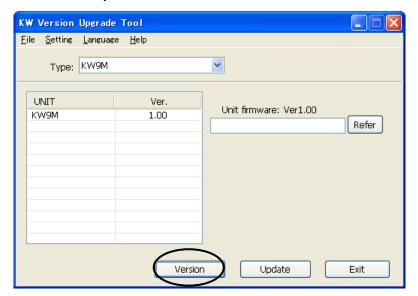
When you have used KW Version Upgrade Tool before, it displays the last updated firmware. If the firmware was moved, the error window will be appeared. Select firmware again and update it.
