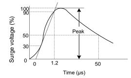
•External noise up to the level shown below is treated as noise voltage, but levels higher than this could lead to malfunctioning or damage to the internal circuit. Although the case is made from fireproof resin, do not mount it next to flammable materials.
