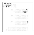
Press <ITEM/ $\triangle$ >, <SHIFT/ $\nabla$ > to set. The setting range differs according to the protocol.
