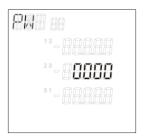
Press <SET> and [0] on the left is blinking. Set password using <ITEM/ $\triangle$ >, <SHIFT/ $\nabla$ >.
